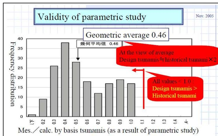
The x-axis of the graph represents the ratio of the scenario tsunami to the simulated design basis tsunami. In all cases, the simulations calculated ratios less than, or equal to, 1, with a median ratio of about 0.46, indicating that the proposed method can be considered conservative and purports to give design values 2 times the scenario basis.
